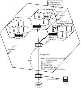
**Figure 4.1 the Architecture of Cellular IP with RSMC** If MN moves from BS1 to BS2, it needs to send a route-update-packet to RSMC during route-update-time.
